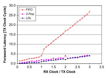
Fig. 15. Latency of two-flop, two-clock FIFO and LDL synchronizers.
