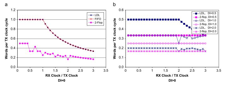
Fig. 18. Throughput comparison for LDL, two-flop and FIFO synchronizers.
