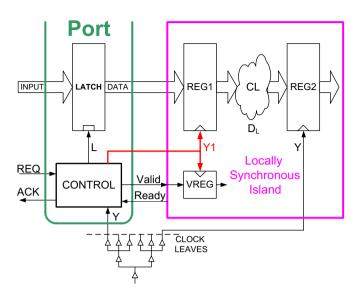
Fig. 5. LDL input port connected to a synchronous island.
