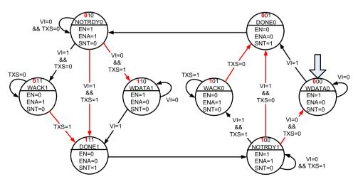
Fig. 2. TX FSM of the fast two-phase synchronizer.
