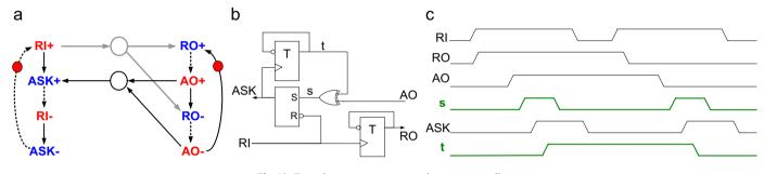
Fig. 10. Two-phase output-port asynchronous controller.
