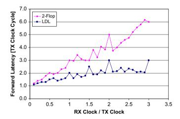
Fig. 16. Latency of *LDL* and two-flop synchronizers for 1.0 · *TX-CLK* interconnect delay.
