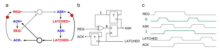
Fig. 8. Two-phase input-port asynchronous controller.
