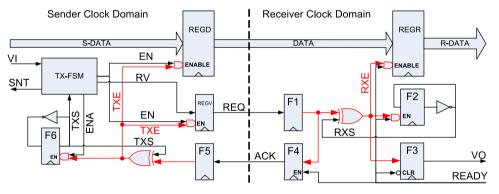
Fig. 1. Fast two-flip-flop two-phase synchronizer.
