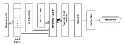
Figure 3. Transmitter architecture in the micro-modem concept
