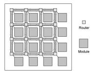
Figure 1. Typical Network on Chip structure.
