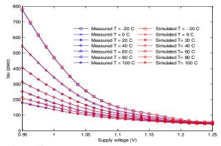
Figure 12. τ Measurements and simulation results versus supply voltage for different temperatures.
