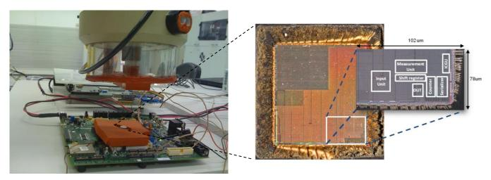
Figure 11. (a) Board including on-chip measurement circuit with thermo stream temperature system. (b) Micrograph of the metastability measurement circuit fabricated in 65nm CMOS
