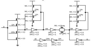
Figure 4. Library flip-flop used for simulations and measurements.
