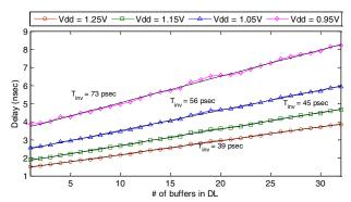
Figure 3. Delay line delay versus number of buffers for different supply voltages at T=20C.  $T_{inv}$  estimated for each curve is shown.
