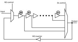
Figure 2. Delay line circuit schematics and RO inverter.
