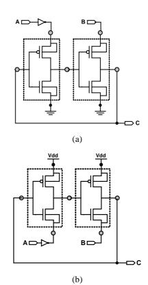
Fig. 6. GDI SR-Latch circuits using (a) F1, (b) F2 functions
