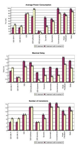
Fig. 9. Simulation results for the C-element implementations
