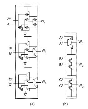
Fig. 19. ORN subnet Full Adder (a) CMOS based (b) GDI based
