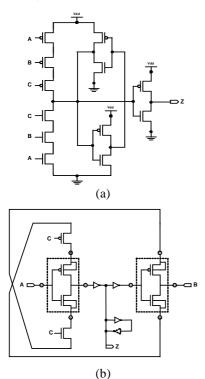
Fig. 4. Three-input C-elements in (a) CMOS and (b) GDI
