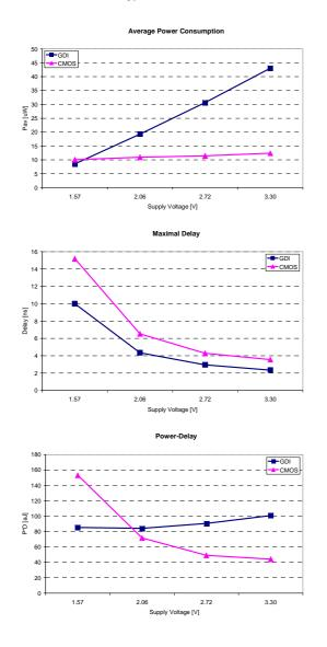
Fig. 10. Simulation results of operation at various supply voltages of 3-input C-element.
