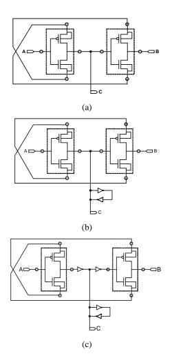
*Fig. 3. GDI implementations of C-element: (a) dynamic, (b) static, (c) buffered static*
