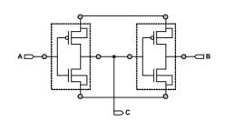
Fig. 7. GDI implementations of dynamic C-element with inverted input A.
