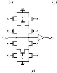
Fig. 2. CMOS C-element Circuits: (a) dynamic, (b) conventional, (c) weak feedback, (d) static, (e) symmetric.
