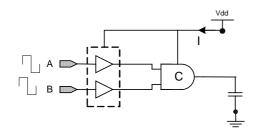
Fig. 8. Simulation environment of C-element.
