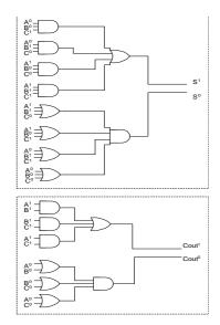
Fig. 20. DRN subnet Full Adder; each gate may be implemented with either CMOS or GDI
