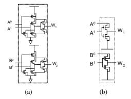
Fig. 15. ORN subnet (a) CMOS based (b) GDI based
